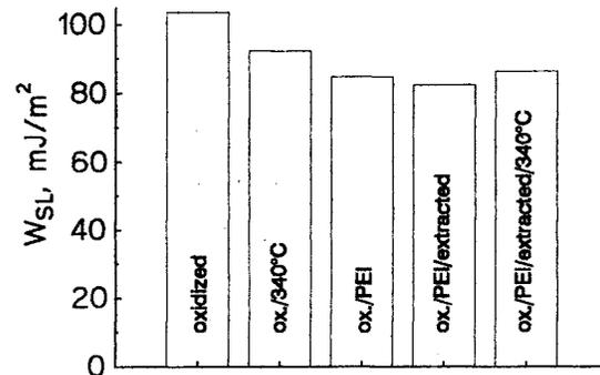
Fig. 2:  $W_{SL}$  with water on various glass like carbon samples; after coating with PEI the sample was treated at 340°C in argon.
