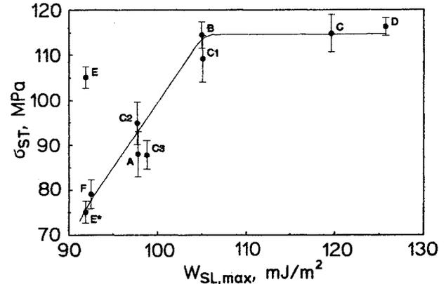
Fig. 1:  $\sigma_{ST}$  in dependence of  $W_{SL,max}$  ( $W_{SL}$  of an aqueous solution with pH = 13) at the carbon fibre surface.
