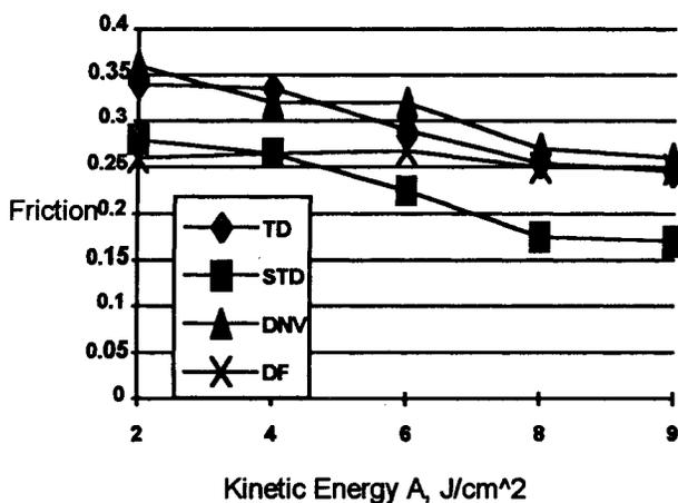
Figure 1. The Effect of Kinetic Energy on Friction.
