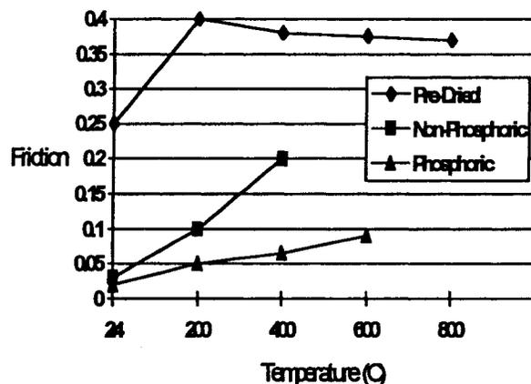
Figure 2. The Effect of Contamination on Friction
