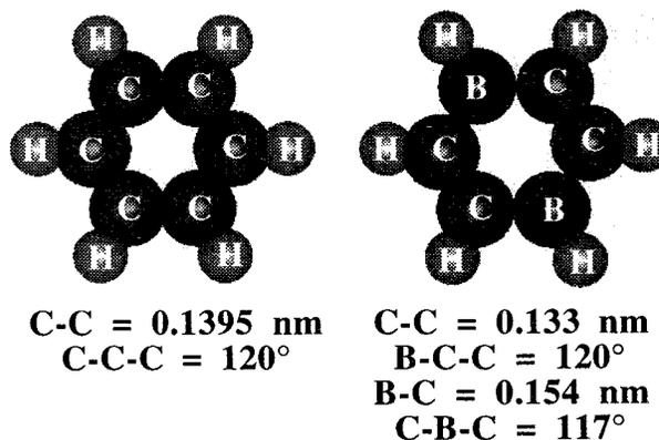
Figure 1 - Computer generated structure of a) Benzene host molecule, b) Benzene host molecule with two borons substituted onto carbon sites.
