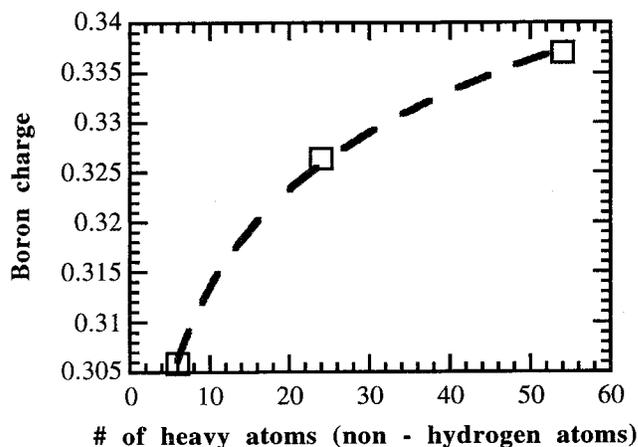
Figure 3 - Charge on boron atoms as a function of the number of heavy atoms (non - hydrogen atoms) in a particular molecule.
